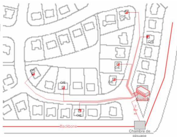
Figure 3.8 : architecture en double étoile active (AON)
