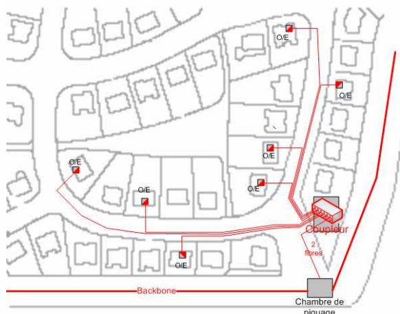
Figure 3.10 : architecture FTTH PON
